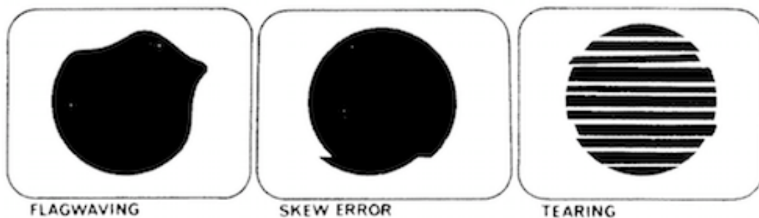
Figure 2 – Time base errors. 9
