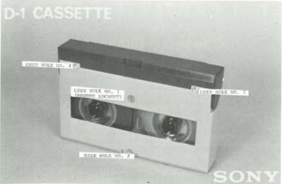
Fig. 5. SMPTE D-1 "S" cassette showing user holes.
