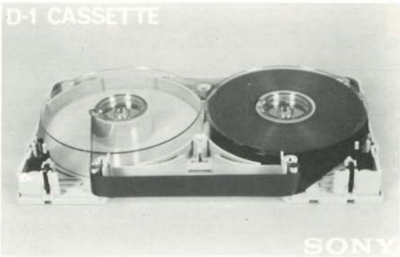
Fig. 7. SMPTE D-1 cassette — internal construction.
