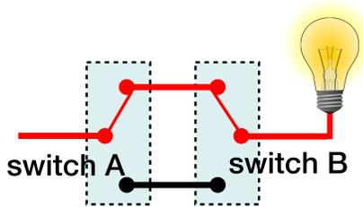
Fig. 1: Both switches are up
