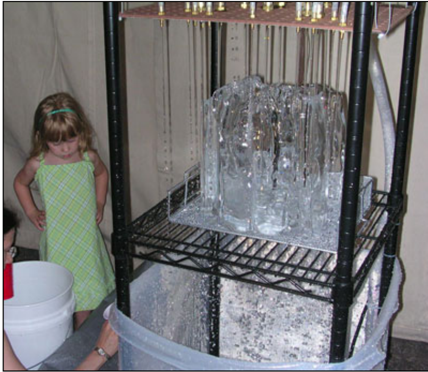
Figure 4. "Automated Architecture Robot" by Ira Spool and Anna Tsy-pin, uses water to sculpt architectural models out of large blocks of ice.
